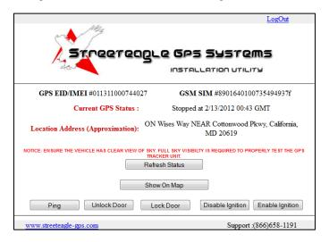
The vehicle status screen will allow you to test proper installation and function of you Vehicle tracking unit though the following options.
